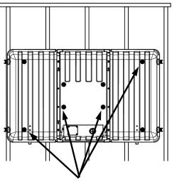
Mounting Holes Do Not Align with Studs
