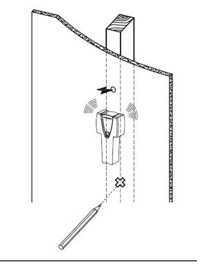
If the wall material is outdoor siding (vinyl or aluminum), stucco, or brick veneer: the wood studs may be difficult to locate with a stud finder due to several layers of construction cladding. You may need to locate the wood stud from the inside wall and use measurements to locate the wood stud on the outdoor wall.
