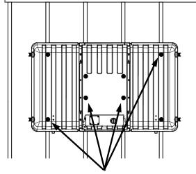
Mounting Holes Align with Studs
