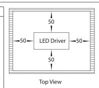
Minimum 50mm spacing needed around LED Driver. LED Driver cannot be covered, If covered warranty will be voided.
