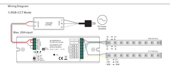
$Note: please\ make\ sure\ the\ dip\ switches\ are\ at\ position\ for\ RGB+CCT\ mode\ as\ shown\ in\ above\ diagram.$
