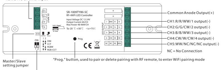
Dial switch for device mode selection, DIM, CCT, RGBW and RGB+CCT 4 modes are available, factory default is RGB+CCT mode
