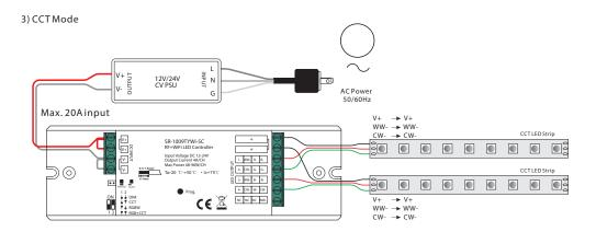
$Note: please\ make\ sure\ the\ dial\ switches\ are\ at\ position\ for\ CCT\ mode\ as\ shown\ in\ above\ diagram.$
