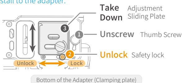
If the camera doesn't have the 1/4-20 screw hole, please put the camera on mount adapter, which has 1/4-20 screw hole, and then mount it following above steps.
