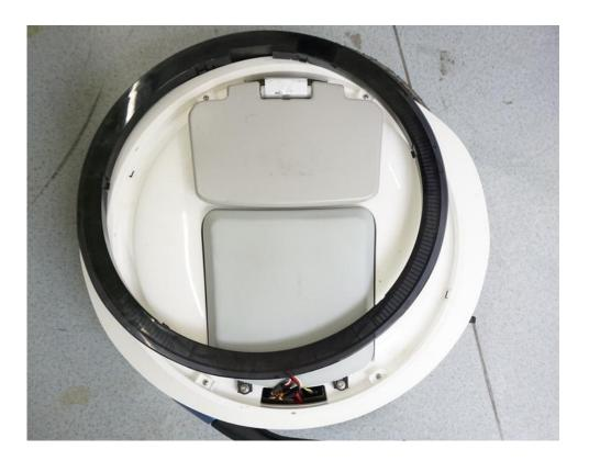
2. The black shell has two LED strips. The front LED strip is connected to the connector marked with "1" and the rear LED strip is connected to the connector marked with "2."
