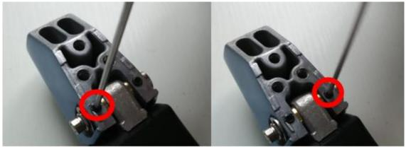
3. Remove the screws directly from the arm and base assembly, then remove the e-clip with side cutters as shown below.
