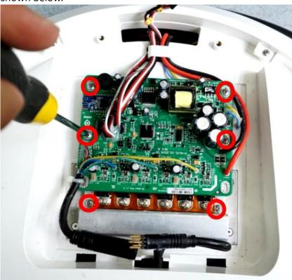
4. After removing the screws, disconnect the power wire and take out all the wires from the white protective clip, paying attention to the wiring harness layout.
