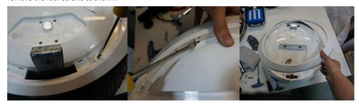
8. Use a 3 mm hex key to remove the casing screws (right side of the Ninebot ONE only) then disconnect the wiring before gently pulling the casing off.
