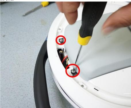
2. Remove the battery compartment cover, paying attention to the wiring harness layout.
