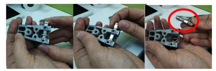
5. Disassembled Handle bar assembly:
