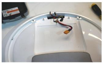
2. Remove the battery (see **Battery Removal**).
