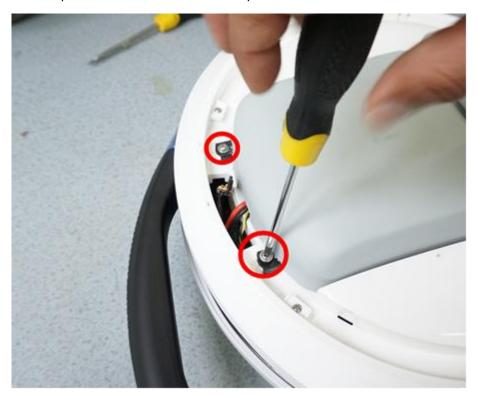
2. Remove the control board compartment cover, then unplug the motor/control board cable.
