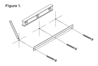
**Step 2:** Install the wall cleat over the dry wall where the 2x4 beam is located.
