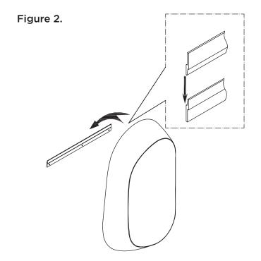
**Step 3:** Place the wall cabinet over the cleat until it is locked into place.
