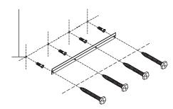
**Step 2:** Measure 30-3/4" (78.2cm) from each pilot hole down and mark the location of the pilot holes for the bottom wall cleat.
