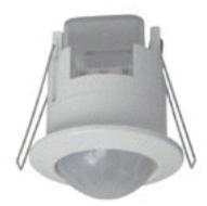
The PIR32 adopts a sensitivity detector and integrated circuit. It gathers automatism, conveniently and safely saving energy with practical functions. Is designed to automatically turn lights on when motion and body heat is detected. It utilizes the infrared energy from humans as a control-signal source; it can start the load at once when one enters the detection field. It can identify between day and night, easy to install and has a wide variety of uses.
