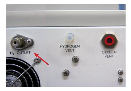
3. Remove the caps from the Oxygen and the Hydrogen vents.
