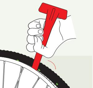
As you are locking pins into place, be sure to tuck in the tire edge into the rim as you go so that the tire sits flush in the rim channel. This will ensure a safe and smooth rolling tire.
