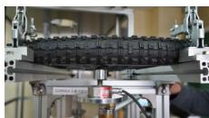
This test checks how much force (cornering and side impact) applied to the side of the tire when the insert is inserted.
