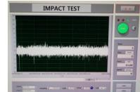
This test calculates the amount of impact the shock sensor receives at the bottom of the tester by dropping the impact weight at 1 meter height. By inserting the insert pieces on top of the sensor, you can see how much impact the insert absorbs.
