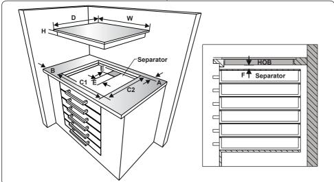
Apply the supplied one-sided selfadhesive sealing tape all the way around the lower edge of the cooktop. Do not stretch the tape.
