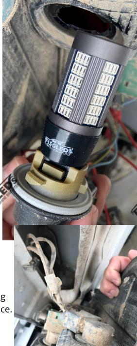
Reinsert the bulbs back into the housing using a clockwise turn to lock it into place.
