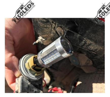
**STEP 5** Reinsert the bulb back into the housing using a clockwise turn to lock it into place.
