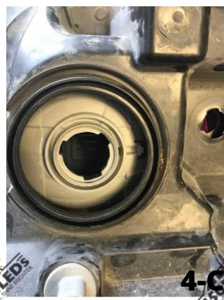
Once your bulbs are installed, slide your rubber seal over your bulb and secure it back into place to seal your headlights.
