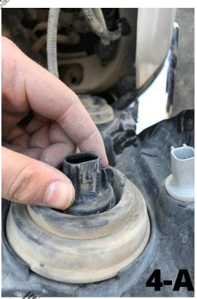
Now that the harness is disconnected from the bulb give the bulb a counterclockwise turn to remove it from your headlight housing.
