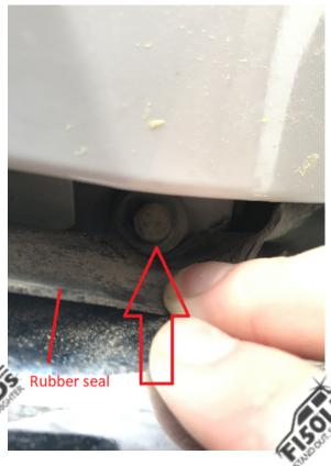
Once these bolts are removed carefully pull your headlight assembly away from your truck. With some moderate force and some finesse the assembly should come right out.
