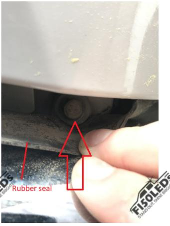
Once these bolts are removed carefully pull your headlight assembly away from your truck. With some moderate force and some finesse, the assembly should come right out exposing your Front Blinker socket.
