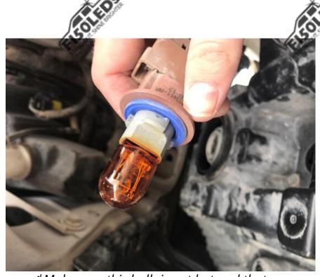
\*Make sure this bulb is not hot and that no power is going to the bulb\*
