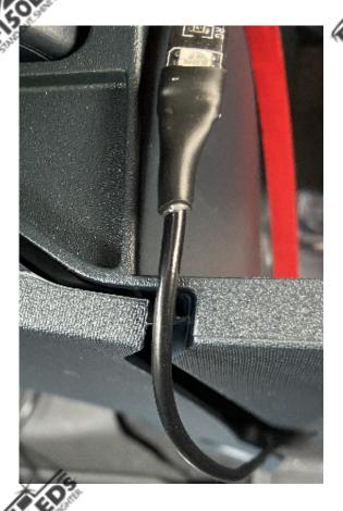
Once the wire is ran into the console pop the plastic trim piece bag into place then reinstall the 10mm bolt.
