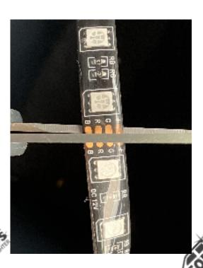
If the LED strip is too long, it can be trimmed with scissors along the copper color part of the strip, once it is trimmed to the correct length mount the strip where you would like in the console.
