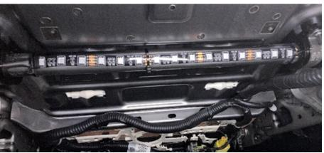
Run the other A wire to the back of the passenger seat and mount it under the elastic straps under the back of the seat.
