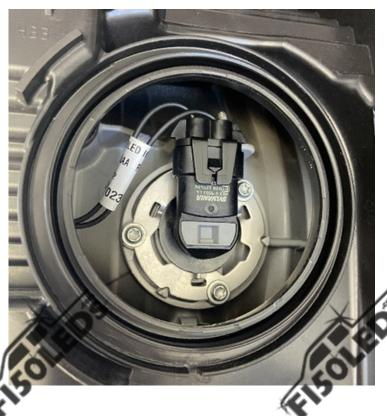
Once the bulb is out of the housing press down on the tab on the connector and release the bulb from the factory wiring. Then connect the ballast to the factory wiring then connect the ballast to the LED bulb.
