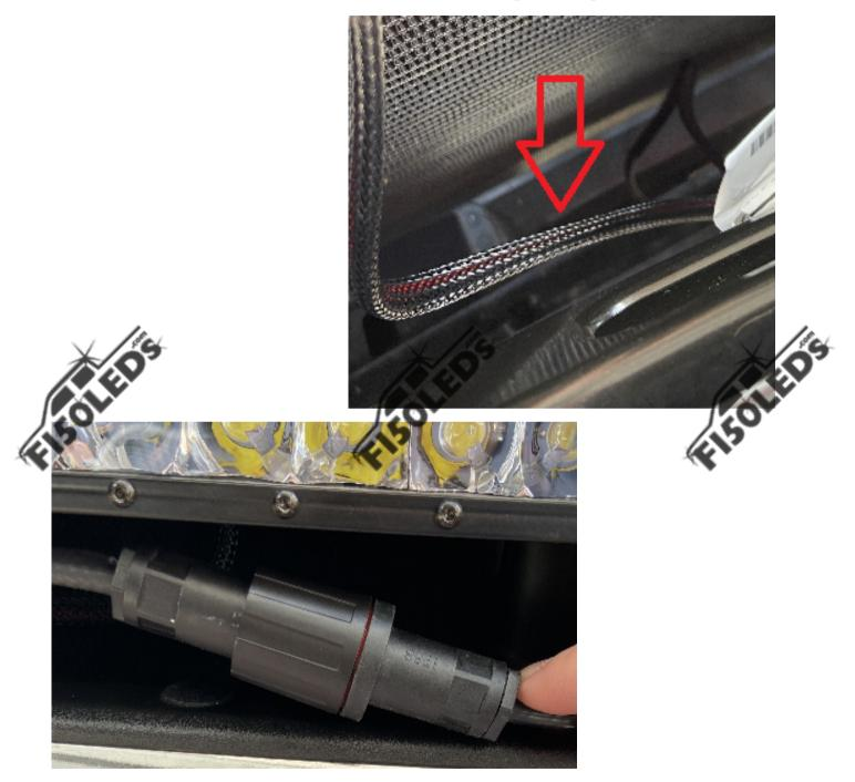
\*Be sure that the wiring harness is zip tied in the engine bay so that the wiring harness does not get caught in any fans or belts. \*
