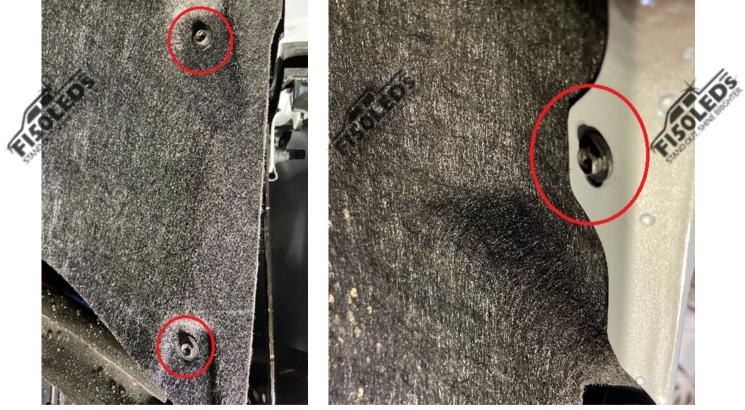
The first two screws are located right inside the wheel well, and the screw connecting the wheel well liner to the trim piece is at the top of the wheel well.
