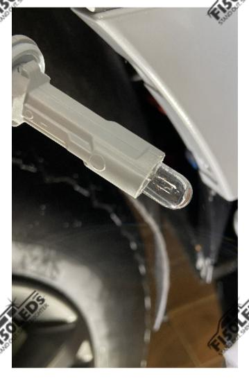
Install your F150LEDS.com Front Marker bulb.
