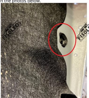
The first two screws are located right inside the wheel well, and the screw connecting the wheel well liner to the trim piece is at the top of the wheel well.
