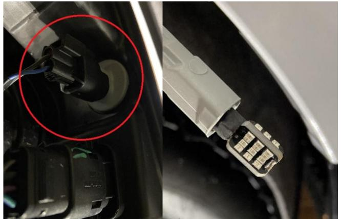
included quick splice connectors to connect the wires from the Raptor kits power harness to the two wires on the front marker socket.
