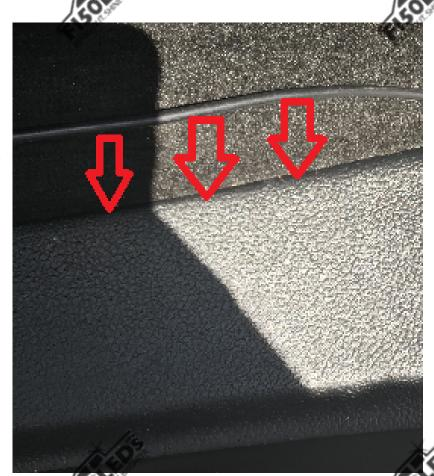
Once the wire is ran to underneath the passenger dash, mount the LED strip to the flat plastic surface at the bottom of the glove box. We recommend tucking the strip under the metal tabs in the photo below to help hold the strip in place.
