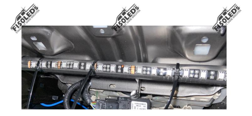
Run the other C wire to the back of the driver's seat and mount it under the elastic straps under the back of the seat.
