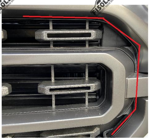
Then run the wire up the grille tucking it where the red line is in the photo so that the wire is not showing hanging in the grille.
