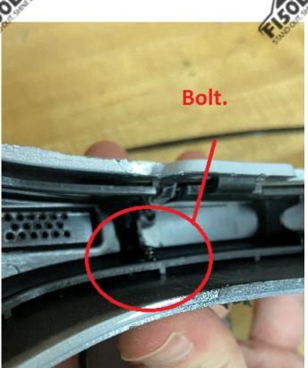
It is a tight opening so we recommend using some needle nose pliers to help be able to work in this tight space.
