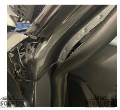
Using a plastic pry tool you can tuck the wire in to the seam shown by the arrows above.
