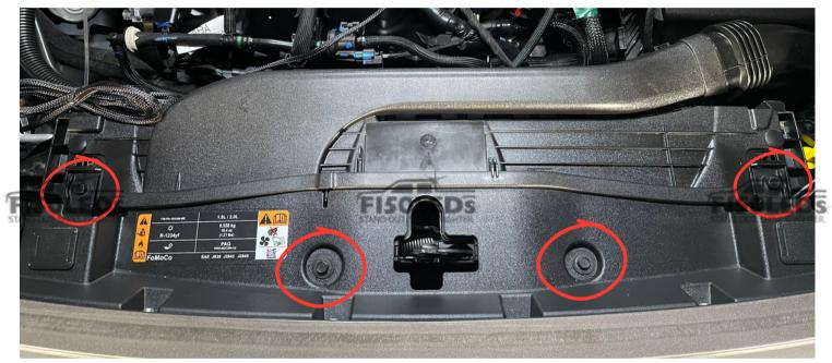
Use a 7mm socket to remove the circled screws
