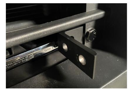
Carefully place a washer, then lock washer, and finally FISOSCREW on the nut. \*BE PATIENT, IF YOU DROP A PART ITSOLEDS WILL BE LOST\*
