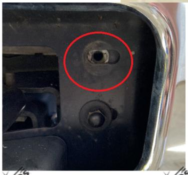
With the bolt in the bracket slide the bolt through the hole show here.
