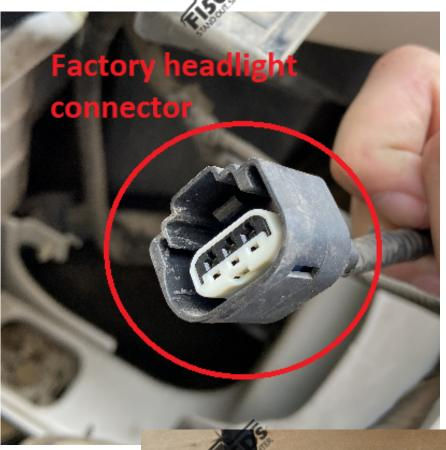
Connect the headlight ballast to the MKV headlight bulb, then plug the ballast into the factory headlight connector, then insert the headlight bulb into the headlight housing and turn it clockwise to lock it into place.
