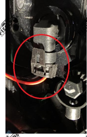
Now take the female end of the fog light resistor and plug it into the MKII Fog light bulb.
