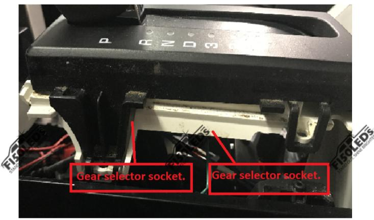
Give the socket a counter clockwise turn to expose the bulb. (Some trucks need to be turned clockwise to expose the bulb).
