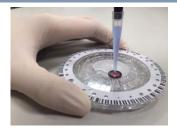
**6.** Use 200  $\mu$ L fixed pipette to draw up 200  $\mu$ L diluted sample, and dispense sample into the reagent disc .
