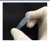
5. Close Eppendorf tube lid after dispensing plasma/serum, slightly shake 10 times to mix plasma/serum with diluent, and centrifuge the sample.
