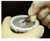
5. Remove the aluminum foil strip covering the sample injection port.
