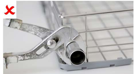
Fig. 5: Removing the central filter without tools
