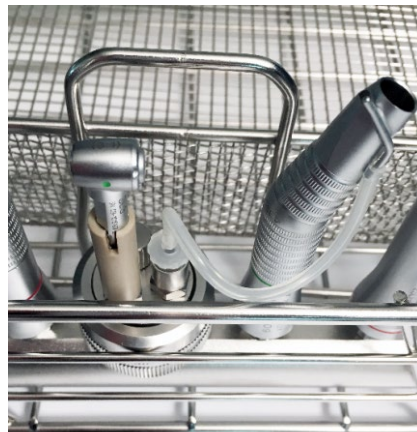
Fig. 35: The adapter is connected with the transfer instrument to be rinsed
