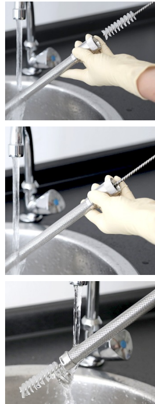
Fig. 38: Cleaning the Cleanfinity filter
