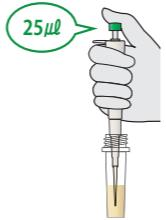
2. Use a 100  $\mu$ l pipette to mix the sample with diluent by pipetting, for 5-6 times.
