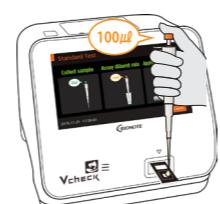
\* If the time to press [START] button is delayed, it may affect the test result.
