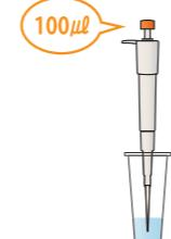
2. Add the mixed sample(100  $\mu$ l) into the sample hole of the test device. Then, press the "Start" button.
