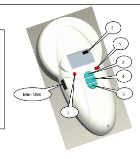
Congratulations, you have just acquired your ISOSCAN2 reader. This reader can read all FDX-B type electronic chips (complying with standard ISO 11784), FDX A chips and HDX chips.
