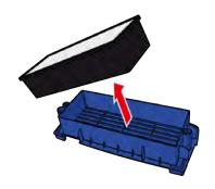
6. Place the replacement filter in the filter cap with the rubber seal facing up.
