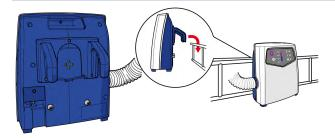
Mounting on a bed rail/end using the bed hooks.
