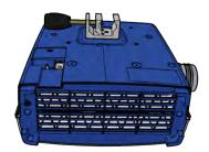
**3.** Remove the 4 M5 screws of the pole clamp using a 4 mm hexagon key and remove the pole clamp.
