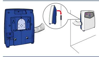
Mounting on a wall using the Wall mount. Release by using the quick-release mechanism.
