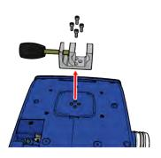
**4.** Attach the Cover at the 3 indicated locations using the first 3 of the 5 M4x16 3 mm hexagon screws with a maximum torque of  $1.5 \pm 0.2$  Nm or  $13.3 \pm 1.3$  in-lb.
