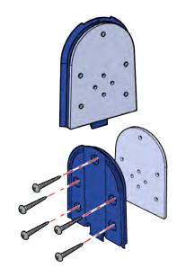
**8.** Optional: Attach the Cover plate to the Wall mount using the 5 M6x6 4 mm hexagon screws. And attach the pole clamp to the Cover plate using the 4 M5 screws which were removed during step 3 using a 4 mm hexagon key.
