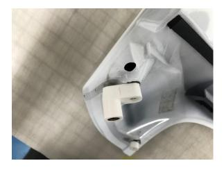
Attach the right and Left side No.1 Marked risers to the wing with the provided 3.5x25 self-tapping screws.
