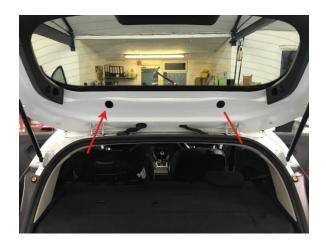
Remove the left and right side wing screws.
