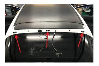
Place the 6 vinyl dot sticker overs the holes that will not be used so that water does not pass into the holes. The picture below will give you the general direction that the risers should be facing prior to placing on to car.
