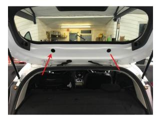
Place the wing on the boot and line the No.2 Central risers with the holes in the boot.
