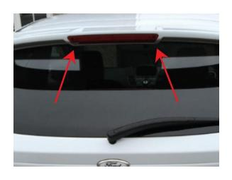
Remove the rear light's screws. Remove the rear light.
