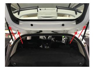
Line up the Right and left side risers with the holes in the boot.
