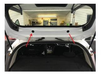
Remove the central wing screws.
