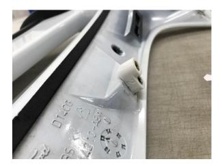
Attach the No.2 Marked risers to the middle part of wing with the provided M6 socket head bolt.
