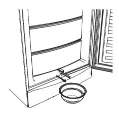
For defrosting pull out the drain water extension over a bowl.
