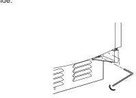
3) Ajustment of the top door: loosen the screws in the hinge above the door, loosen the hinge above the door and turn
