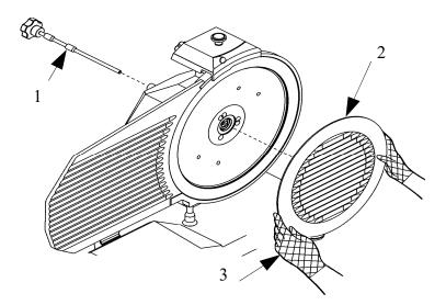
FIG. n°14 - Release of blade guard
