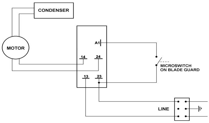
FIG. n°8 - Single-phase electric system arrangement - Schalter Profi
