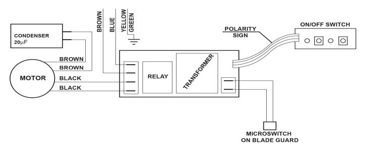
FIG. n°6 - Single-phase electric system arrangement
