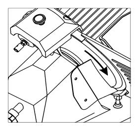
FIG. n°5 - Sense of blade rotation
