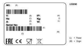
FIG. n.4 - Technical-serial number plaque
