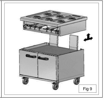
Once the appliance assemblies are in situ they can be re-assembled The oven pipe connections must be soundness checked for a leak free joints. A bubble spray method may be employed.
