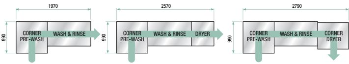
Indicates direction of operation (dirty to clean). All Minirack Evolution models can be ordered running in either direction but must be specified at time of order. Only R3010 and R3020 without additional modules can be reversed once ordered.
