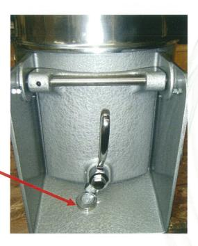
3. Retighten nut to secure door cam once correct position has been established.
