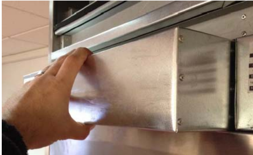
Sliding the Stage 3 Filter Panel Forward
