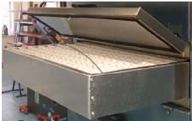
Opening the Access Panel and Removing the Stage 2 filter
