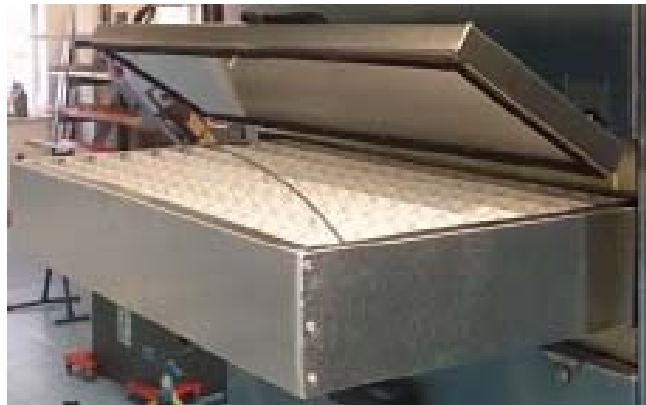
Opening the Access Panel and Replacing the Stage 2 filter
