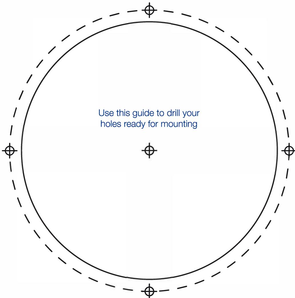
*NB if you do not wish to use the drill plan, ensure the central tube hole is a diameter of 119mm and 4 x 4.2 fixing holes are located at 90 degrees apart around the circumference.*
