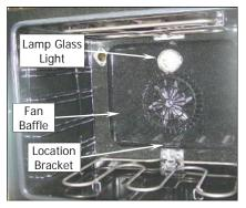
b. Whilst holding the fan baffle in place, undo the lamp glass (anti-clockwise) and remove.
