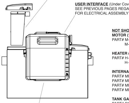
**GREASE/OILS COLLECTION CONTAINER** FOR W-200-IS THROUGH W-500-IS USE PART# GC-10
