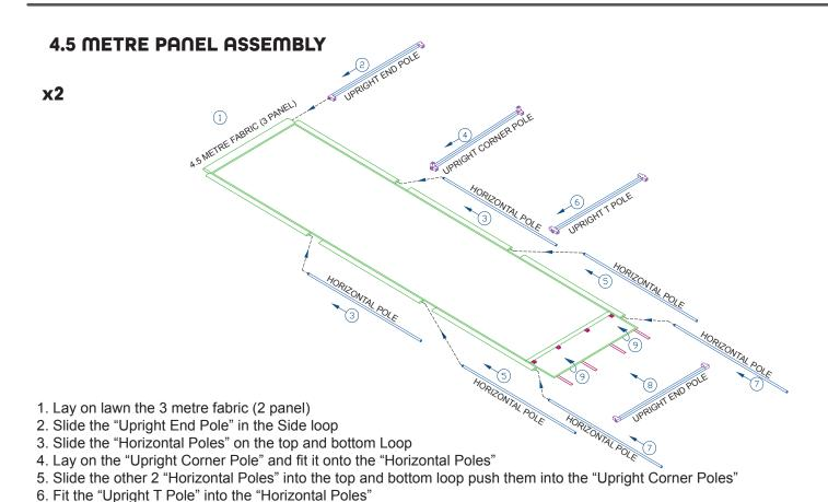
7. Slide the other 2 "Horizontal Poles" into the top and bottom loop push them into the "Upright T Poles"
