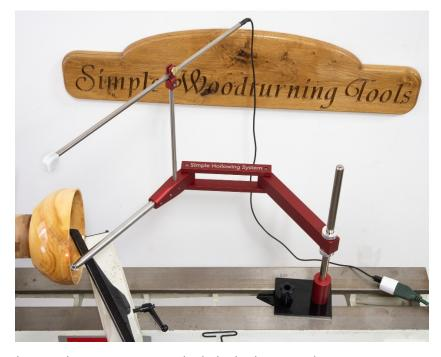
1. Clamp the mounting base and main pivot pin to the lathe bed. Secure the main pivot pin to the mounting base with an Allen set screw.
