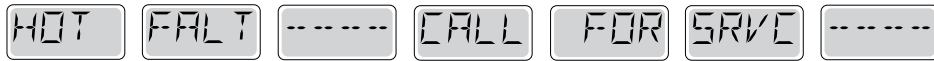
A Pump Appears to have been Stuck ON when spa was last powered UP
